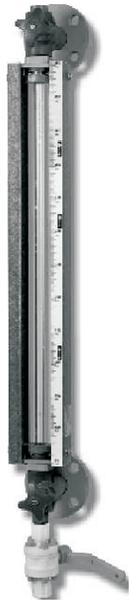
Gauge is fitted between two end fittings through gland packing. The gauge is mounted parallel to tank so as to form a close loop causing tank liquid to seek its level in the gauge. The Gauge Glass is protected with 'C' channel. End fitting has built-in isolating valve, drain valve & vent plug.
