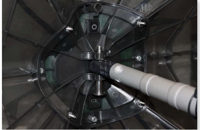
When using the short pole or with the SAH adapter base kit for canvas hoods, the stationary pole adapter should be used to keep the hood pole from pivoting. Place the stationary pole adapter onto the SAH and attach using the screws and wing nuts provided (below). Once secure to the SAH, insert the short pole and secure in place using the locking pin.
