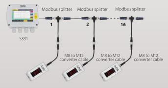
**Remark:** The S331 can maximum provide 10 W power to the connected devices. If more power is required a separate power supply is needed.
