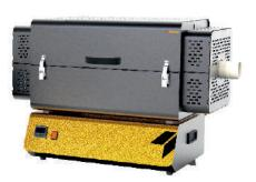
Tempsens Split Tube Furnace has a horizontal oriented chamber with a furnace body that splits into two halves. Ability to open furnace facilitates the operator to change the working tube easily and insers vessels like reactors with flanges which is not possible in non split type furnaces. Working tubes can be easily changed to make the furnace work with variety of tube diameters. Optional features allows user to modify working environment to vacuum or particular gas surrounding (inert gas).
