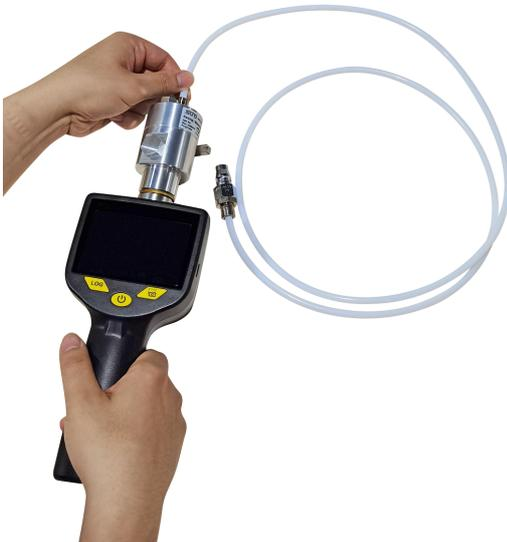
2. Connect the teflon hose to the measuring chamber.
