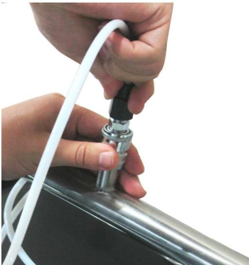
3. Connect the quick coupling at the other end of the teflon hose to the process.
