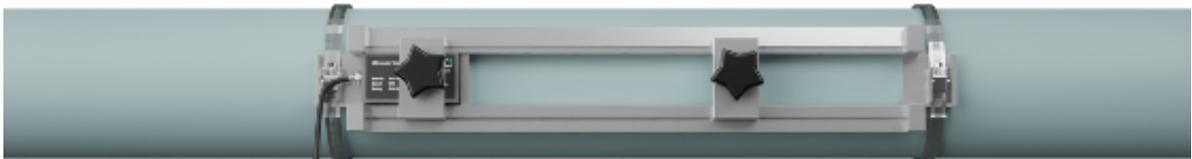
7. Put the other flow transducer from top of the fixture. Make sure that the distance between the two transducers is the "Transducer spacing" value shown on the mobile phone App. Rotate the knob to fix.
