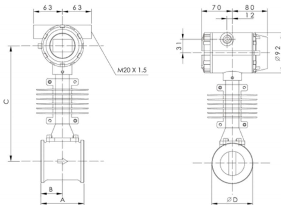
Figure 1 Water Vortex flow meter outline dimensional drawing
