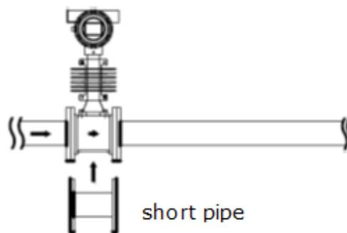
**6.2.3 Wafer type vortex flow meter installation diagram**
