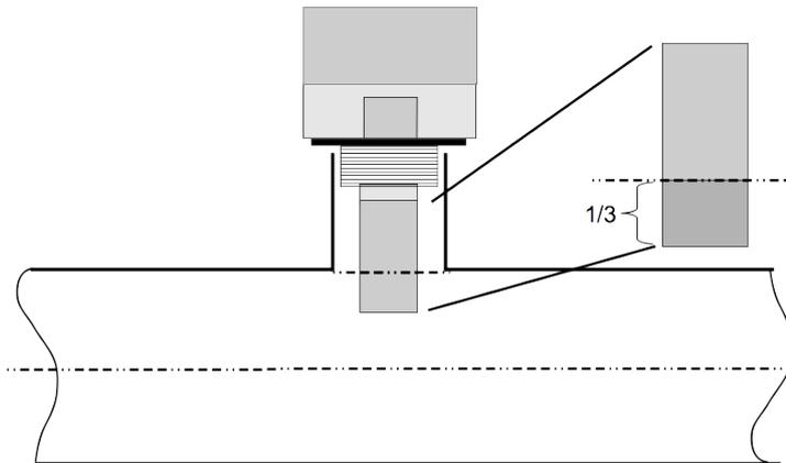
Full flow installation. The sensor is in the pipe.
