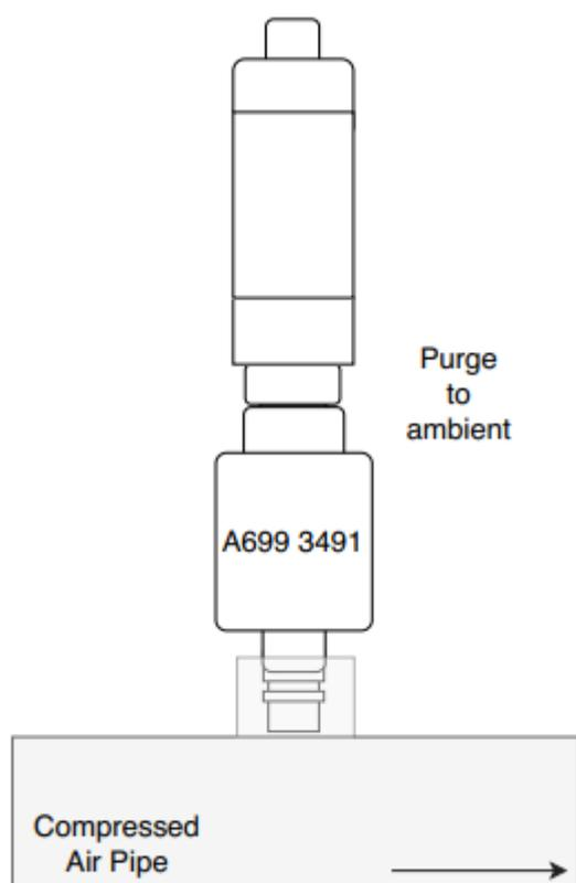
1. Mount the sensor on the measurement chamber by using the G1/2" connection.
