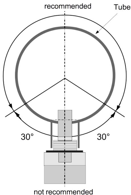
Please install the sensor only in the recommended area like you can see in the picture. A upside down installation is not permitted. Please consider that the distance to the vertical level must be  $>30^\circ$ .
