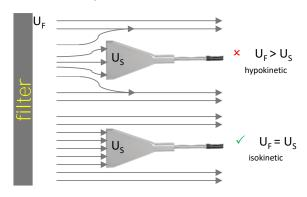
$U_S$ ...flow velocity at probe inlet  $U_F$ ...flow velocity from the filter
