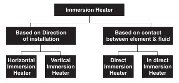
**Direct Immersion Heater:** An Electric Heater bundle in which the heating elements will directly immerse into the fluid to be heated are known as direct immersion Heaters.
