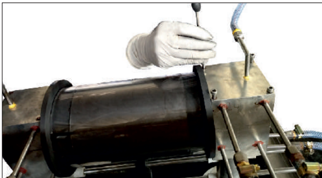
Slide back the copper block and reattach the allen key bolts with the spanner
