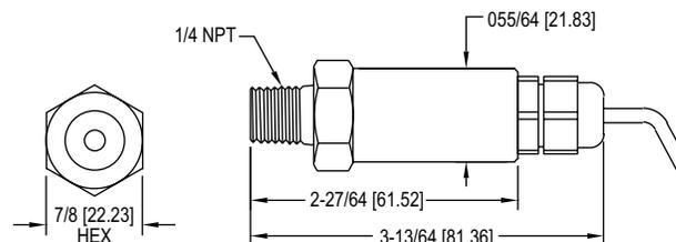
The **Series 626 & 628 Pressure Transmitters** converts a single positive pressure into a standard 4-20 mA output signal. The Series 626 and 628 can be used to accurately measure compatible gases and liquids; Series 626 full scale accuracy is 0.25%; Series 628 full scale accuracy is 1.0% (see specifications). Designed for industrial environments with a NEMA 4X (IP66) housing, this transmitter resists most effects of shock and vibration.
