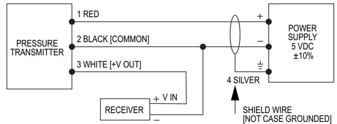
Figure G: Voltage output connection
