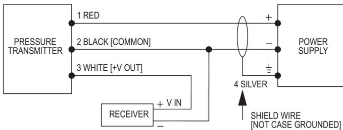
Figure D: Voltage output connection
