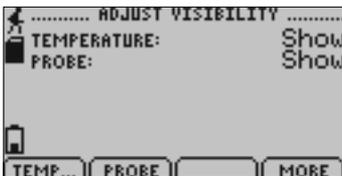
*Displays options for changing the viewing of both channels on the main screen (either shows a particular channel or hides it.)*
