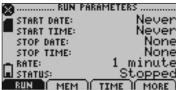
*Displays information about run parameters including date of recording start (start date), time of recording start (start time), stop date, stop time, recording rate, and current status.*
