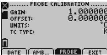
*Displays calibration information for external probe channel.*
