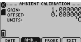
*Displays calibration information for internal temperature channel.*
