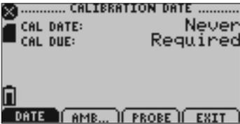
*Displays date of last calibration and due date of next calibration.*
