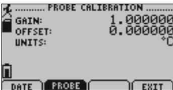
*Displays calibration information for temperature channel.*
