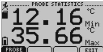
*Displays statistics (Maximum recorded value, Minimum recorded value, and average recorded value) based on channel (External Probe)*
