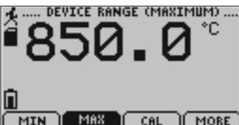
*Displays values indicating maximum external probe data detectable by the DLI-R.*
