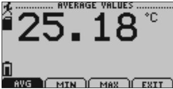
*Displays statistics from the channel (External Probe) sorted by type (maximum recorded value, minimum recorded value, or average value).*
