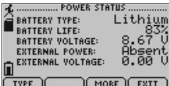
*Displays details about power available to the device including the battery type, battery voltage, and external voltage.*
