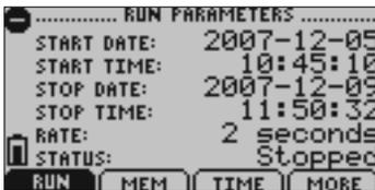
*Displays information about run parameters including date of recording start (start date), time of recording start (start time), stop date, stop time, recording rate, and current status.*
