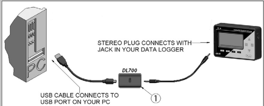
1. Insert the USB connector of the DL700 into an available USB port. Fully insert male connector of the DL700 interface cable into the female receptacle of the data logger\*.
