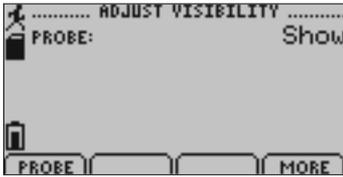
*Displays options for changing the viewing of the channel on the main screen (either shows the channel or hides it.)*
