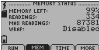
*Displays information about the device's memory capabilities including percent of memory available (memory left), number of readings taken so far (readings), max number of readings (max readings), and wrap.*
