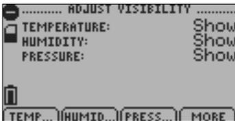
*Displays options for changing the viewing of the three channels on the main screen (either shows a particular channel or hides it.)*
