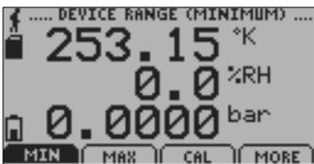
Displays values indicating minimum temperature, pressure and humidity detectable by the DLI-P.
