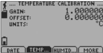
*Displays calibration information for temperature channel.*
