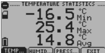
*Displays statistics (Maximum recorded value, Minimum recorded value, and average recorded value) based on channel (Temperature, Humidity, or Pressure).*
