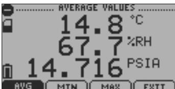
*Displays statistics from all 3 channels (Temperature, Humidity, and Pressure) sorted by type (maximum recorded value, minimum recorded value, or average value).*
