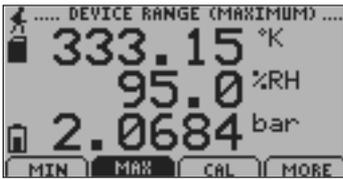
*Displays values indicating maximum temperature, pressure and humidity detectable by the DLI-P.*
