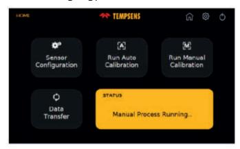
**Sensor Configuration:** In this screen user select the sensors Thermocouple (J, K, B, N, R, S, T type) / RTD (PT 100, PT 1000, PT50 etc.) for calibration with their serial number and temperature unit (C/F/K).
