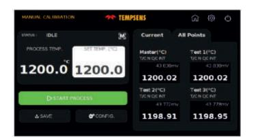
**Auto Mode:** In this screen user sets the temperature Points for calibration (Max 5 Points)
