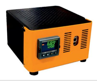
CAL FAST offers medium temperature range from -10°C to 120°C. It is a highly stable standard furnace for calibrating thermocouples / RTD. The comparison volume is a metallic block of aluminum, which has diameter of 6.5mm and 8.5mm and 110mm long. The temperature of the calibrator is set and controlled by a self tuned PID controller with automatic super fine adjustment
