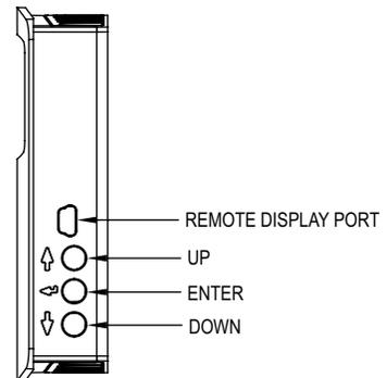
Figure 5: Side view of transmitter
