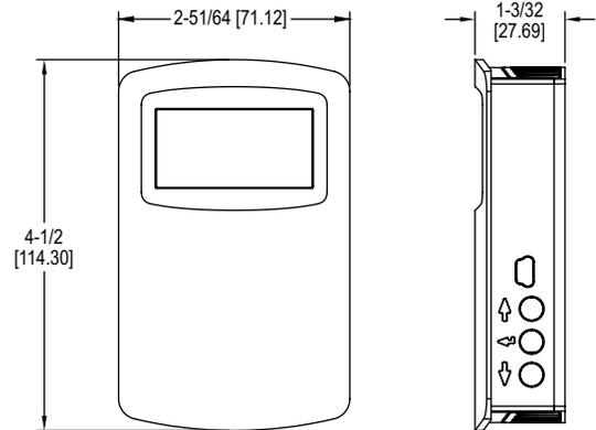
Series CDT and CDTR Wall Mount Carbon Dioxide Temperature Transmitters accurately monitor the CO<sub>2</sub> concentration and temperature in schools, office buildings, and other indoor environments to help achieve LEED® certification. Additionally, the Series CDTR also measures ambient relative humidity. In order to achieve a higher level of accuracy, the Series CDT includes digital barometric pressure adjustment.
