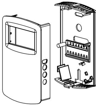
Figure 1: Removal of cover from back plate
