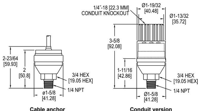
The low cost **Series 673 Pressure Transmitter** is a fixed range transmitter designed for harsh environments and suitable for high shock and vibration applications. Constructed of stainless steel, the Series 673 provides a 4-20 mA output signal with 0.25% accuracy. Use the Series 673 in industrial OEM equipment, hydraulic systems, HVAC equipment, industrial engines and compressor controls.
