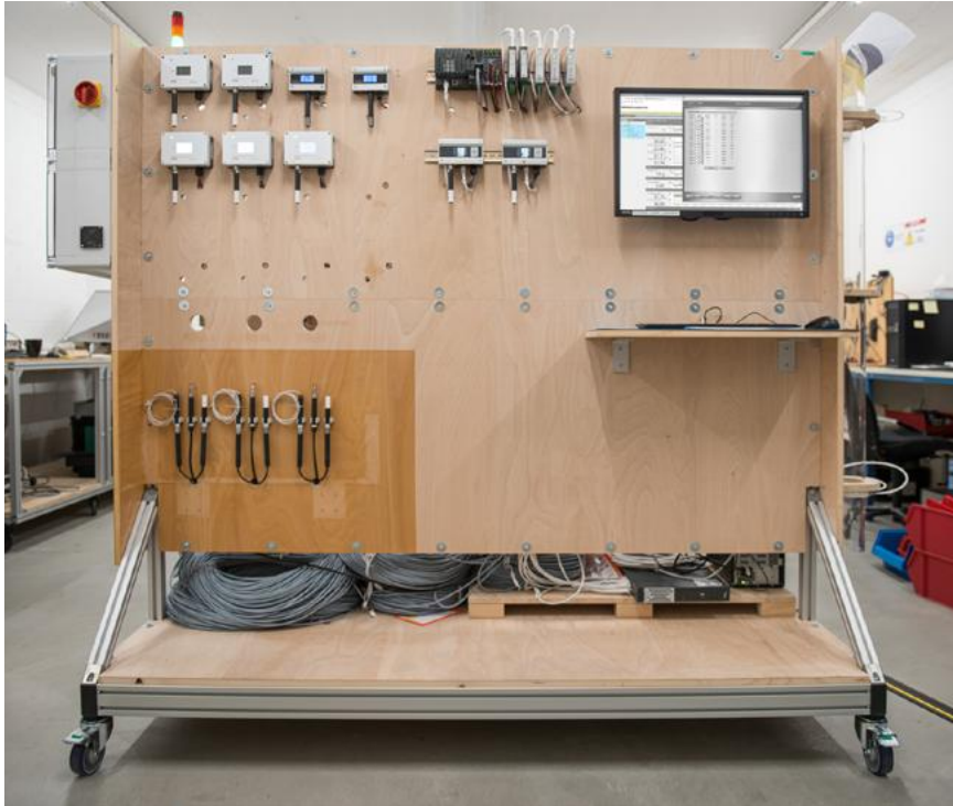
Rotronic Modbus application wall
